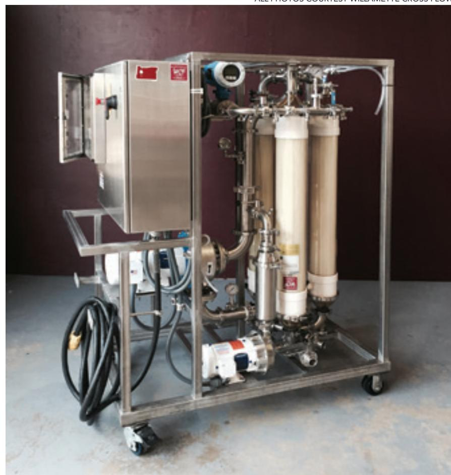
Designed for the smaller winery, the WCF filter is compact and highly portable throughout the cellar.
