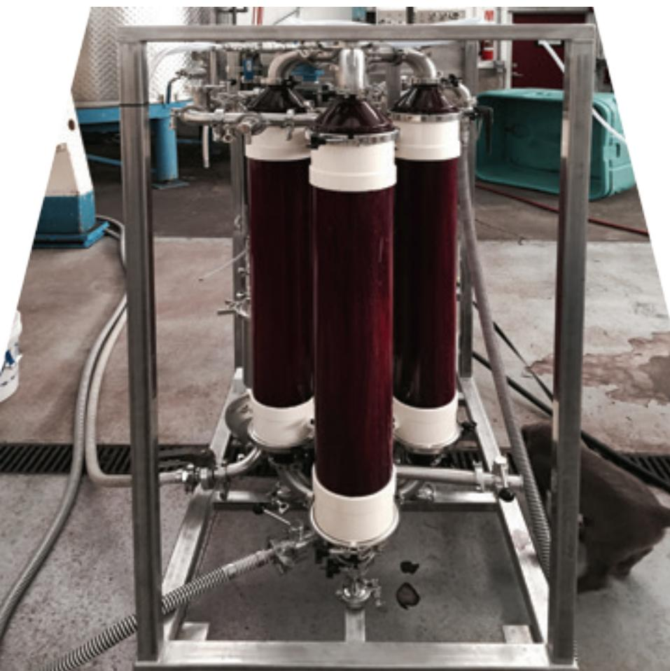
The patented, symmetrical, three-cartridge manifold provides even flow and pressure across all filtering media.
